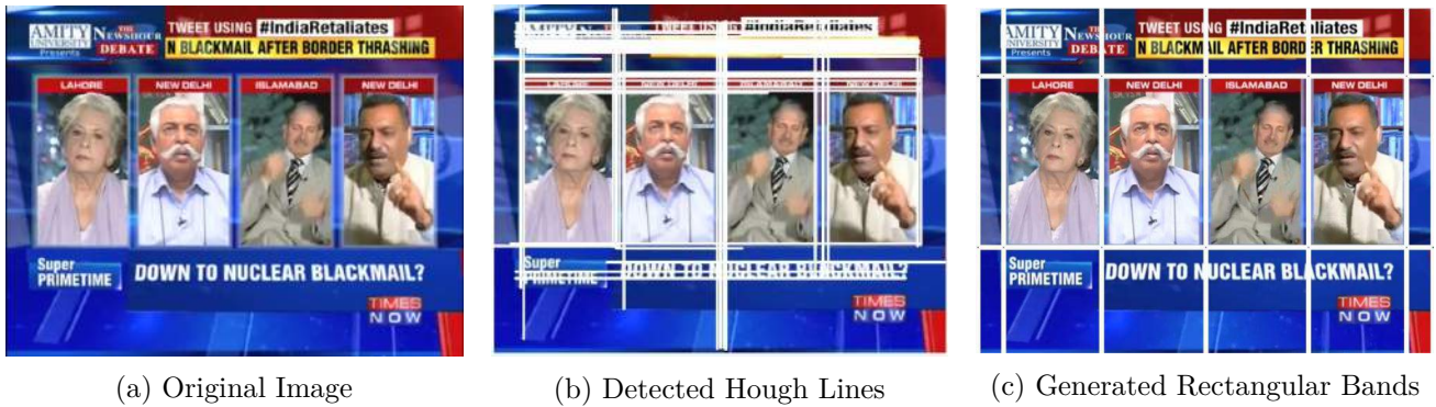
Figure 3.1: Output of Progressive Probabilistic Hough Transform
